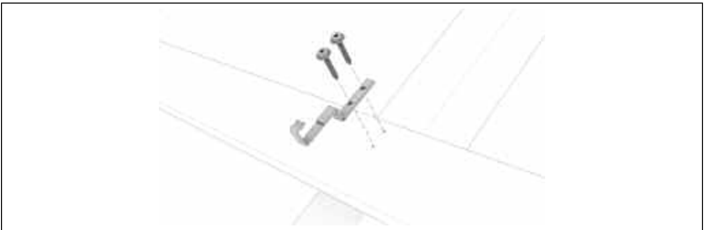
Image 3-3: Mounting clamp “profile”
