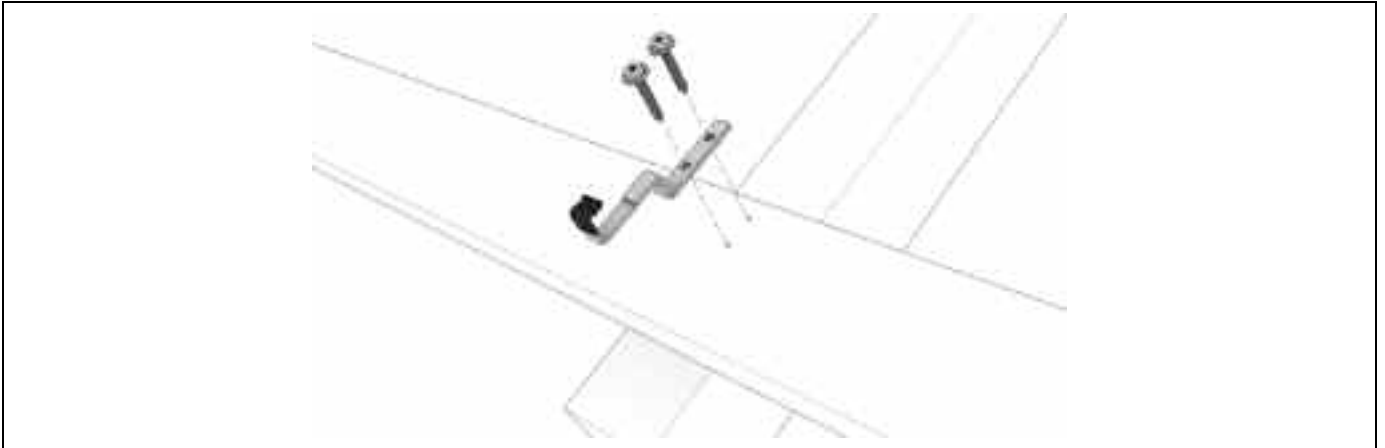
Image 3-4: Mounting clamp "glass"
